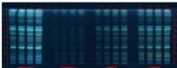
Fig.1: UV-366 nm :Treated with Vanillin / Sulfuric acid
